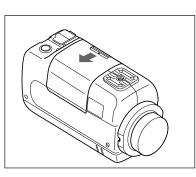
**2** To open the battery compartment cover, slide the cover in the direction indicated by the arrow.
