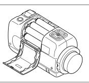
• To close the cover, insert the protrusions on the cover in to the holes on the battery compartment on the instrument, and then press the cover in until it clicks.
